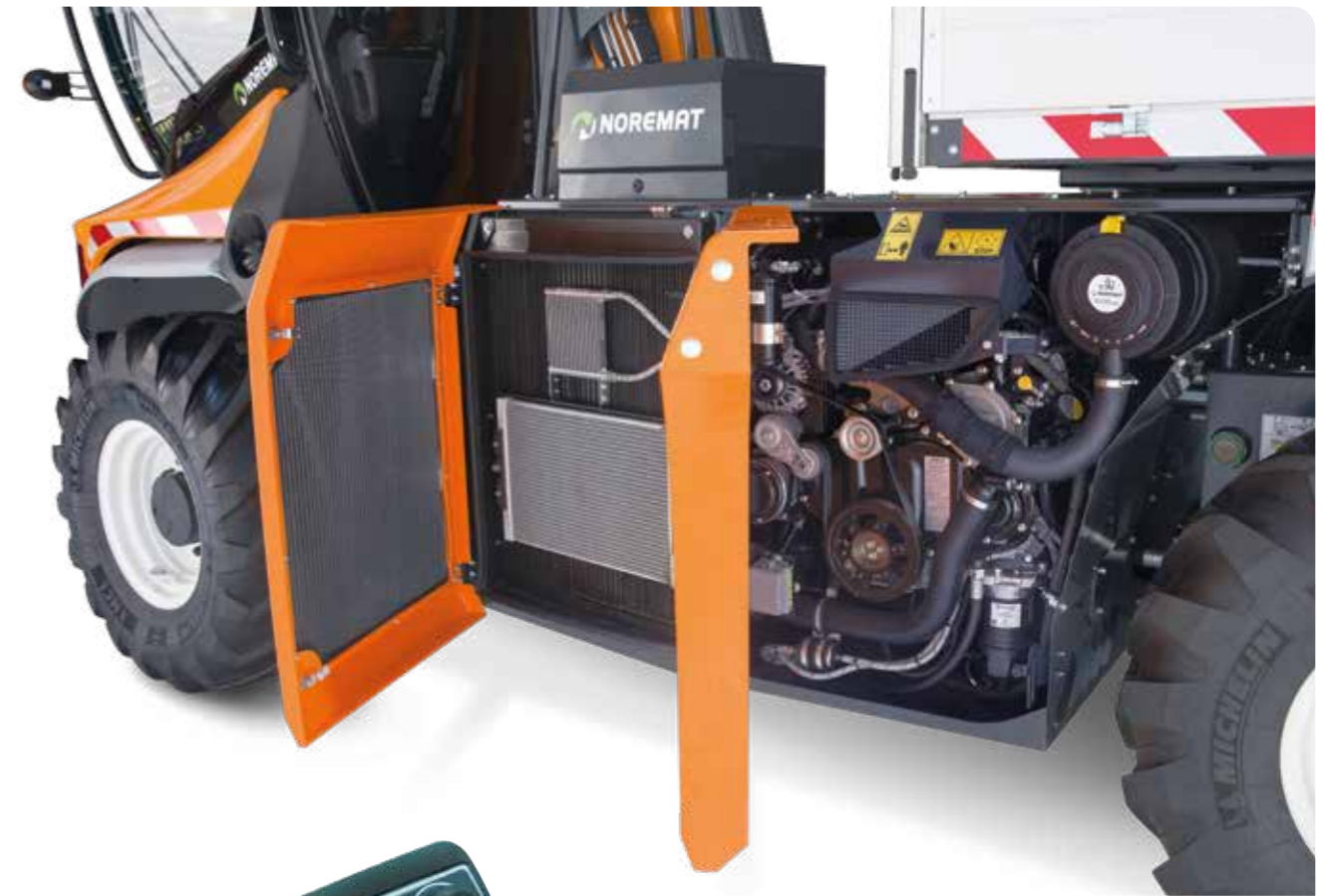
Hinged covers for immediate access to engine and cooler compartments
